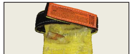
Internal Rod Damage If Internal Rods are visible, damaged, cracked, broken or distorted, remove from service.
