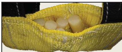
Broken Stitching If stitching is broken and no longer separates and/or encapsulates the Internal Rods, remove from service.
