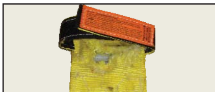
Cuts, Tears and Punctures If CornerMax® Pads have been damaged, they will no longer provide protection and must be removed from service.
