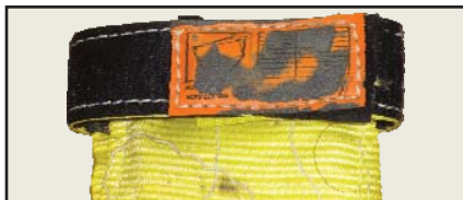
Damaged, Missing or Illegible Tag The tag must include: Name or Trademark of Manufacturer, Stock Number, Protection Capacity and Use/Safety Information.
