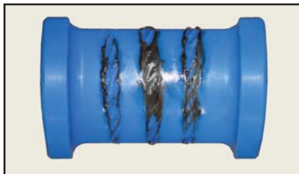
Structural Damage If Magnetic Corner Protectors are damaged, remove from Service.
