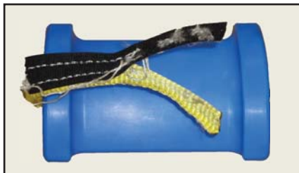
Damaged Retaining Straps If Retaining Straps are missing, damaged or non-operational, remove from service.
