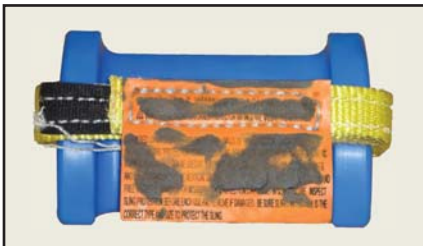
Damaged, Missing or Illegible Tag The tag must include: Name or Trademark of the Manufacturer, Stock Number, Protection Capacity and Use/Safety Information.
