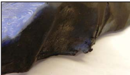
Temperature or Chemical Damage Do not use at or allow exposure to temperatures above 194° F (90° C) or below -20° F (-29° C). Ensure chemical compatibility BEFORE use.
