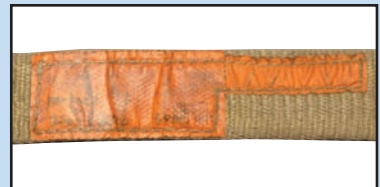
MISSING OR ILLEGIBLE TAG
