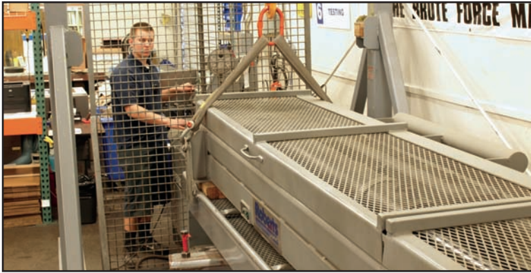
Our 600,000 pound test machine will accommodate sling lengths up to 120 ft.
