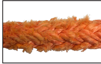
Excessive External Abrasion
