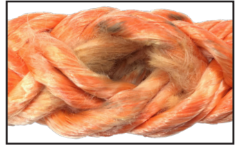
Excessive Internal Abrasion
