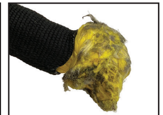
Damage to the Knot
