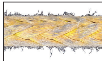
Excessive External Abrasion
