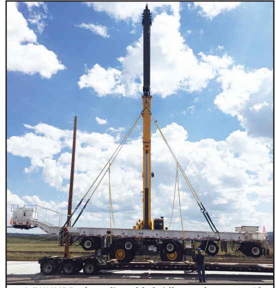
1-1/2" UHMPE 4-leg adjustable bridle rated @ 91,800 Lbs.
