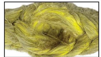
Excessive Internal Abrasion
