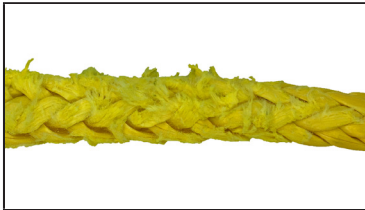
Excessive Wear & Abrasion
