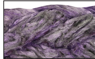
Excessive External Abrasion
