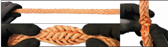
Internal abrasion may be determined by pulling one strand away from other strands to inspect for powder, broken filaments or volume reduction.
