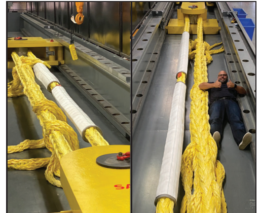
5" Endless Rope being pulled to 200% Proof Test. 1.23 Million Lbs.
