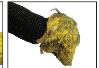
Damage to the Knot
