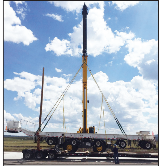
1-1/2" UHMPE 4-leg adjustable bridle rated @ 91,800 Lbs.
