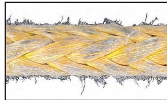
Excessive External Abrasion
