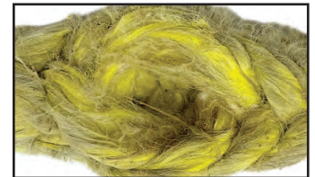
Excessive Internal Abrasion
