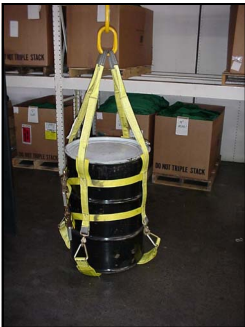
Step 3: Set drum on bottom support bridle and attach to top assembly hooks.
