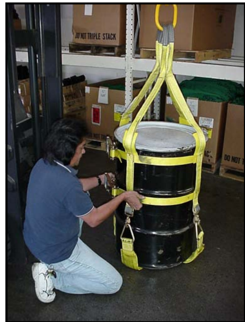
Step 4: Lift load just enough to clear the ground. Lower and re-adjust bands, if necessary. Repeat the above step until balance and control are achieved.
