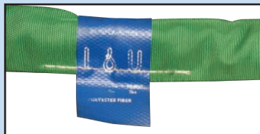
MISSING OR ILLEGIBLE TAG
