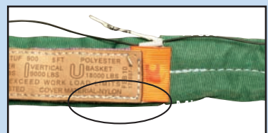
TATTLE TAIL MISSING (Sling fails)
