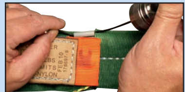
FIBER OPTIC (Lack of light transfer - Sling Fails)
