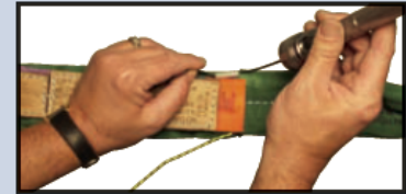
FIBER OPTIC-No Light Transfer (Sling fails inspection)
