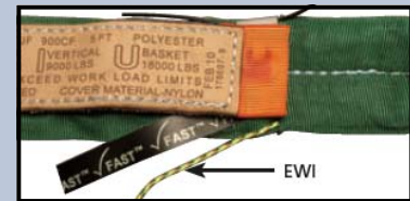
EXTERNAL WARNING INDICATOR ✓CHECK FAST® EWI PRESENT (Sling passes ✓Check Fast® Criteria)
