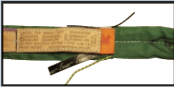
✓CHECK-FAST® EWI PRESENT (Sling passes inspection)
