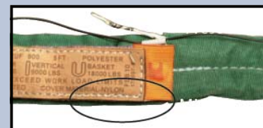
TATTLE TAIL MISSING (Sling fails)
