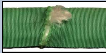
CUT OR DAMAGED YARNS
