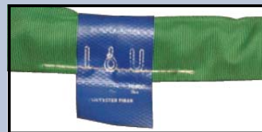
MISSING OR ILLEGIBLE TAG
