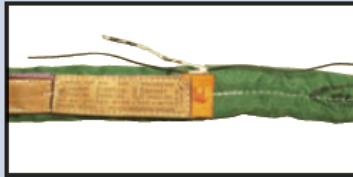
TATTLE TAIL MISSING (Sling fails inspection)
