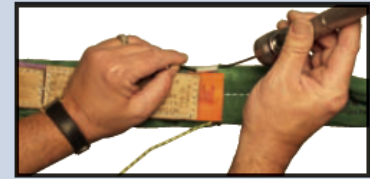
FIBER OPTIC-Transfers Light (Sling passes inspection)
