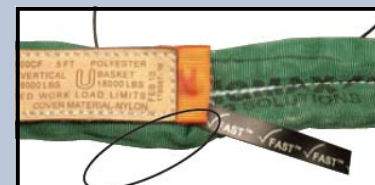
EWI MISSING (Sling fails ✓Check Fast® Criteria)
