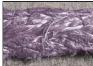
Excessive Wear & Abrasion
