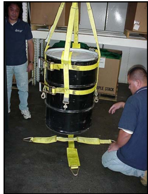
Step 2: Lift drum just enough to pass bottom support under drum.
