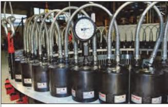
Blade bearing connection using ITH-Multi-tensioning system
