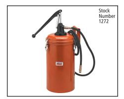
Quality built Lincoln Bucket Pumps dispense high-pressure lubrication at temperatures as low as 0° F / -18° C. Large lubricant capacity with easy pumping action develops a 3,500 PSI maximum pressure to lubricate closely fitted bearings. Automatic pressure release prevents nozzle drip, waste and mess. Pump and lid assembly easily removes as a single unit for filling.
