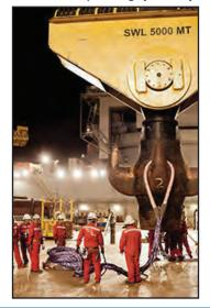
If possible, place the splice over the lift or connection point to allow for equalized elongation in the UHMPE Endless Rope Sling body members.
