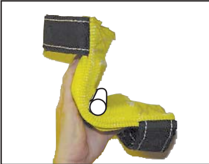
A “TUNNEL” IS FORMED BETWEEN THE PAD AND LOAD EDGE
