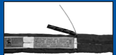
✓FAST™ RIBBON AND EWI EXTEND FROM COVER (Sling passes ✓FAST™ Criteria)
